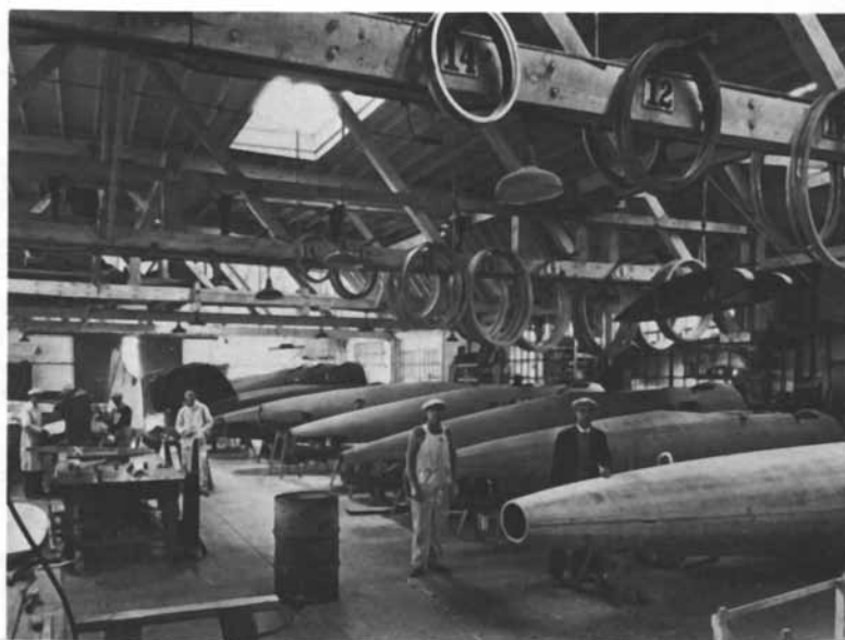
Figure 2. The Lockheed Vega production line, early 1920s. Note the similarity of these bonded wood structures to aircraft currently being made from aluminum (photo courtesy of Lockheed - California Company).
