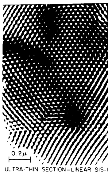
Figure 1. Transmission electron micrograph of a styrene-isoprene-styrene triblock copolymer.
