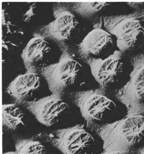
Figure 3. Electron micrograph at 13,000 times magnification showing moisture blush in nitrocellulose lacquer film. Key: SBA, 7.0% w; BUOX, 13.0% w; water: 80.0% w; temp, 25 °C; air flow, 20 l/min. Reproduced with permission from Ref. 38. Copyright 1967 Shell Chemical Co.
